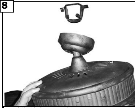
8 Carefully lift fan assembly onto mounting bracket. Rotate fan so that the notch on the ball engages the ridge in the mounting bracket. This will allow hands-free wiring.
